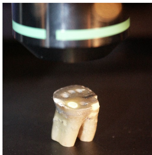
Figure 1. Holes in the specimen, drilled throughout laser scanning for the treatment of hard tooth structure. The volume measurement of the holes lead to the ideal energy distribution for an optimised laser scanning system.
